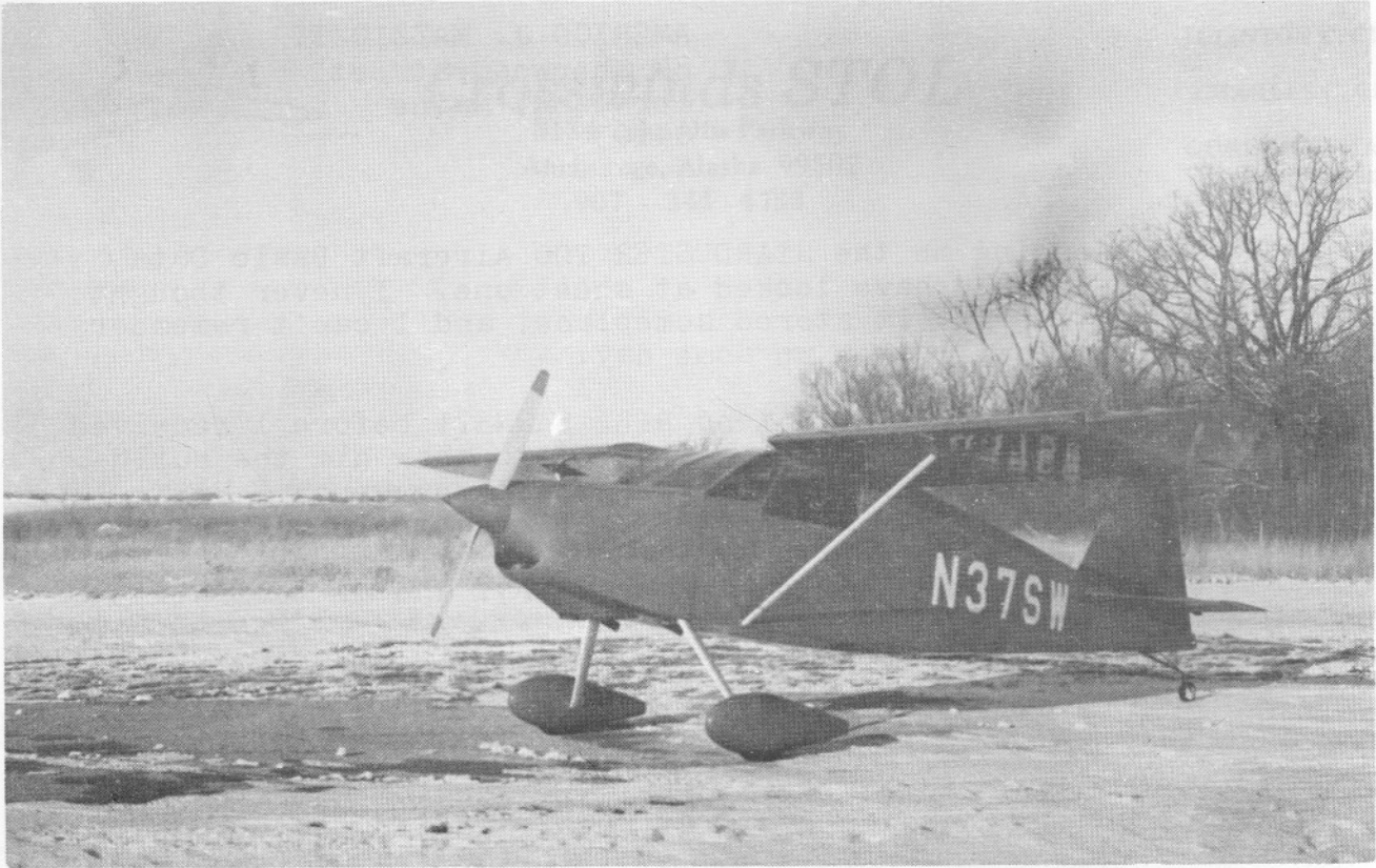
A PICTURE OF STEVE WITTMANS TAILWIND. THIS MACHINE FLIES ON A CONVERTED OLDSMOBILE V-8 ENGINE, AND HITS A LAP SPEED OF 200 MP.H.
