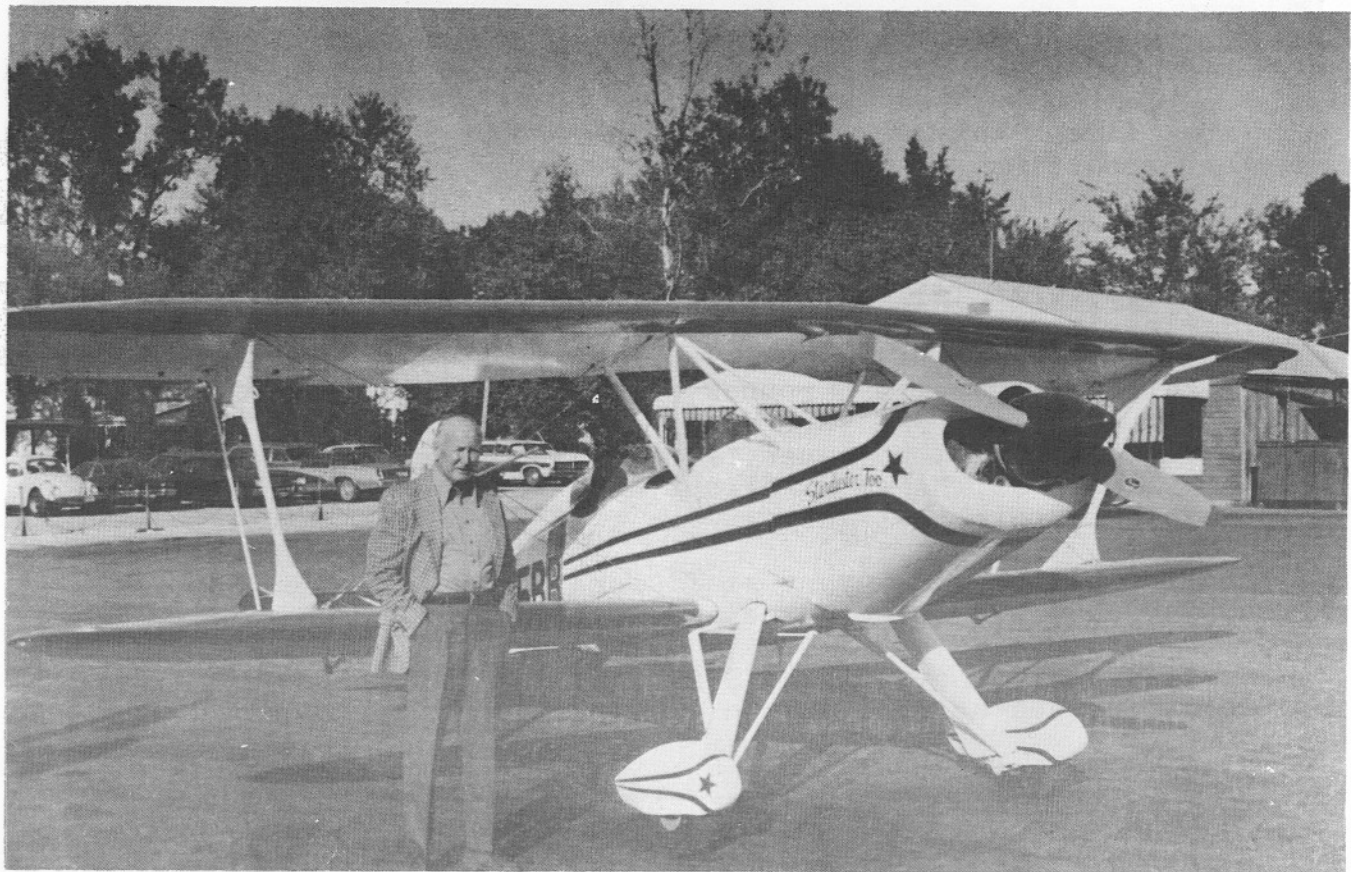
OUTSTANDING STARDUSTER TOO BY JACK BYCRAFT, OF DENFIELD, OTTAWA, CANADA. FEATURES TWO PLACE SLIDING CANOPY AND ALUMINUM GEAR. BELOW IS RAY BRANSON OF KIMBERLY HEIGHTS, MO, WITH HIS SECOND STARDUSTER TOO. RAY'S WORKMANSHIP IS IMPECCABLE.
