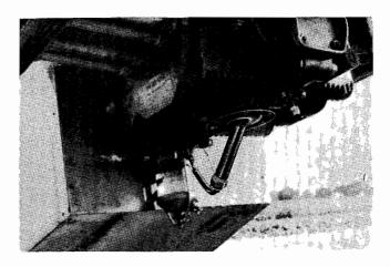
be oiled. This would give the temperature of the oil going into the engine, and this is what is desired. Of course, it is not always possible, so directly in the oil pan is about the next best bet. Also the installation as shown would be subject to cracks at the base of the tube where it fastens to the oil pan. A small brace out near the end of the tube up to the oil pan would be advisable."
